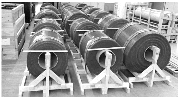
Figure 10: Disposable wooden racks for transporting rolled reinforcement grids
