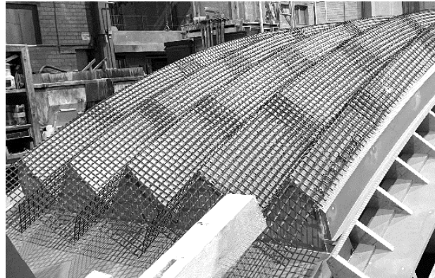
Figure 13: Formed reinforcement grids
